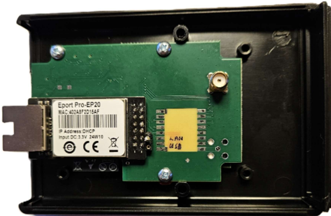
RFX transceiver with 433MHz and Eport LAN controller installed.
